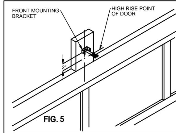
Remove front mounting bracket (See Fig. 1) from rail assembly and install on front wall above spring assembly, Fig. 5. If headroom permits, bottom edge of bracket should be 2 inches above high rise point marked on header. Secure bracket to wall using either lag screws or self tapping screws furnished in hardware package.
