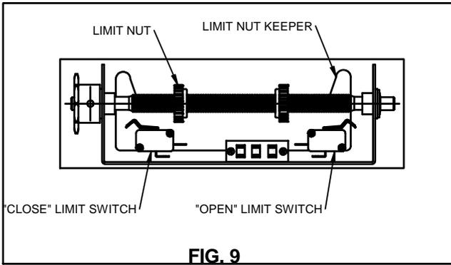
When clutch is properly adjusted, raise door to the full open position and stop door at the desired height and set the open limit nut as described above. After setting limit nuts in desired position, make certain that limit nut keeper is engaged in grooves on limit nuts. When making fine adjustments, turn nut no more than 1/4 turn at a time. To stop door earlier, move limit nut closer to limit switch. To stop door later, move nut away from limit switch.
